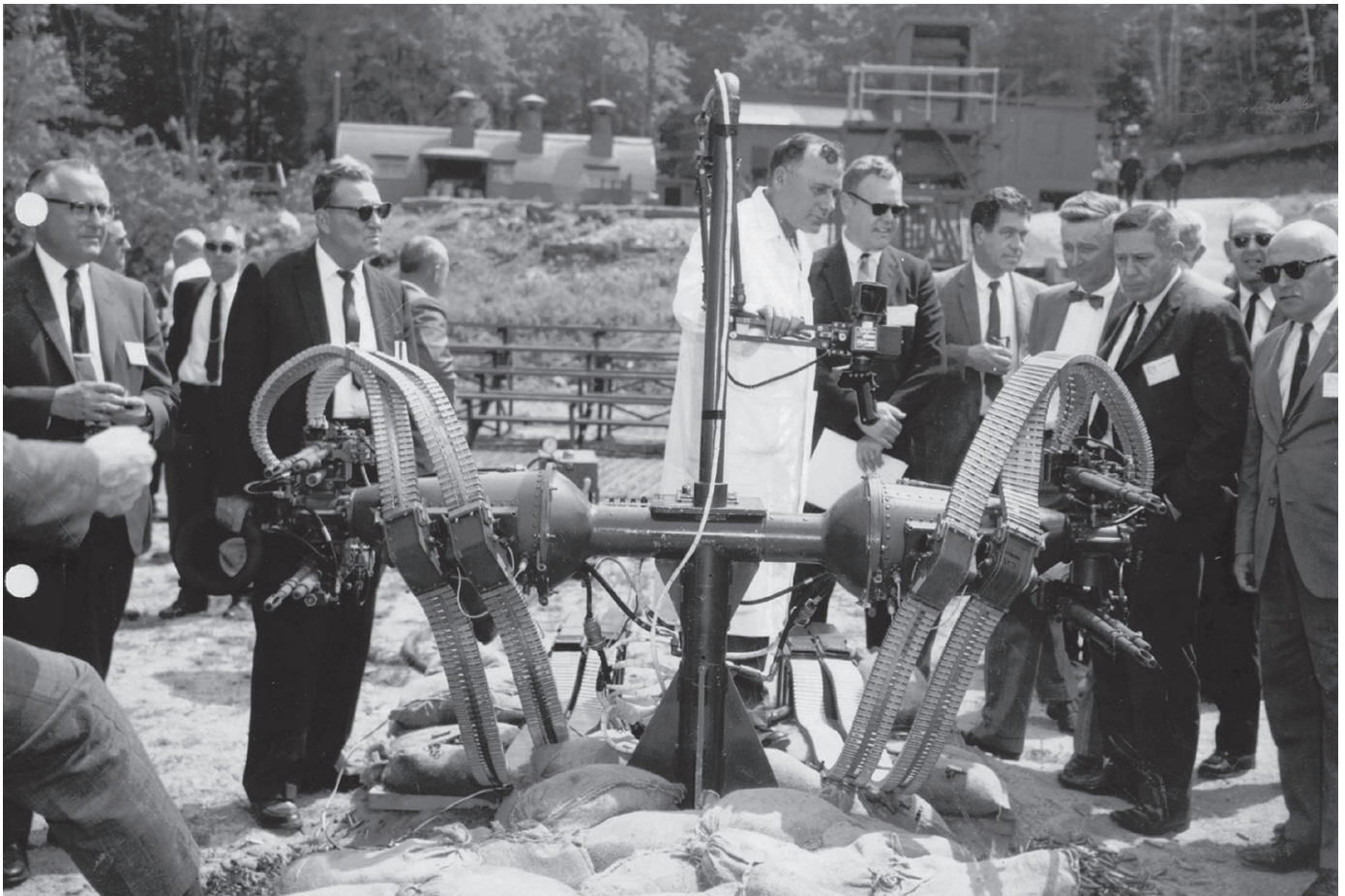
At Quabbin Gate 52, evaluators participate in testing during development of a Vulcan mini gun on a simulated helicopter mount. photo courtesy of Edward T. Knight
