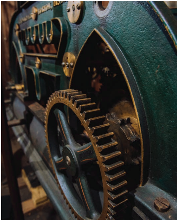
Renovated cleaned and honed Ware bell gears operate the hands that bring chime time back to town. photo © by Dennis Pariseau
